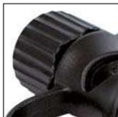
The innovative inseparable quick-action cable retainer allows the cable to be fixed (without using a single screw) by just turning the screw collar, ensuring that any pulling or twisting of the cable will not be transmitted to the ends of the wires connected to the socket connectors or plug pins. This innovative system keeps all water and/or dust out of the product, protecting it from damage.
